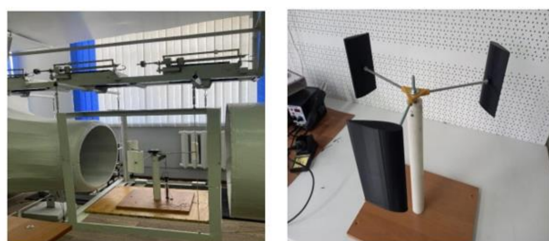
Fig. 1. . Experimental model of a wind turbine with a three-bladed rotor: (a) rotor with modified asymmetric blades (test configuration); (b) rotor with symmetric blades (baseline configuration).
