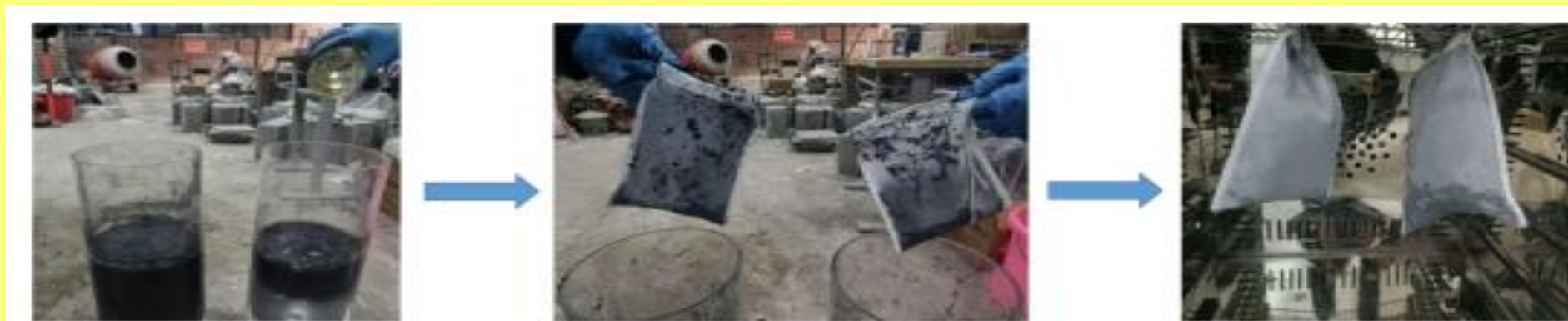
Fig.7 Flow chart of the adsorption experiment of engine oil by EG
