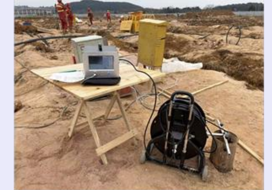
Fig. 6. The smart PIV groundwater measurement system.
