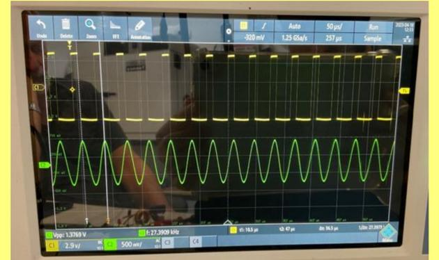
Figure 7 : A stable sinusoidal signal was monitored for a resonance frequency of 27.39 KHz
