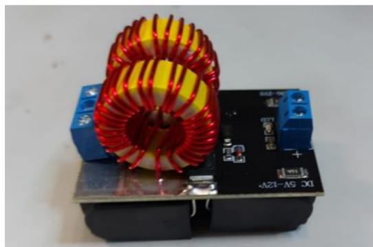
Figure 4 : Illustration of the dedicated transformer which is the main part of the multivibrator.
