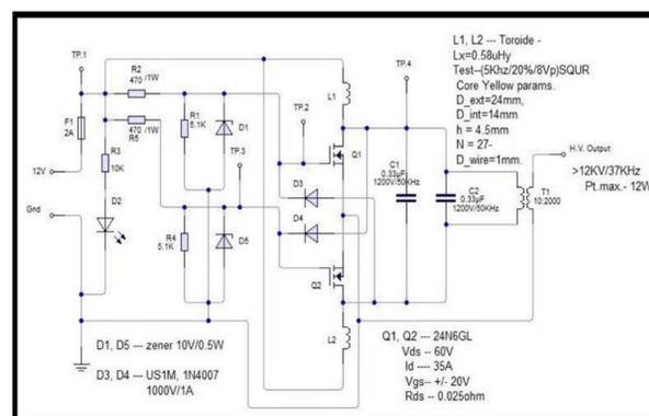
Figure 5 : Schematic of the multivibrator circuit.
