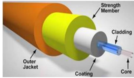
Figure 2 : schematic illustration of the optical fiber. Next is a multivibrator (module 4), which is connected to a high voltage transformer and generates the plasma signal.
