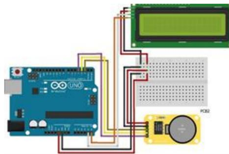
Figure 3 : Schematic of the Arduino circuit.
