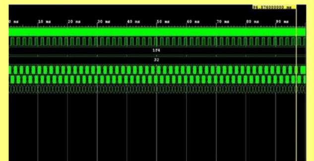
Figure 8 : Simulation data for PMW signal that was produced with 500 Hz and duty cycle of 50%.
