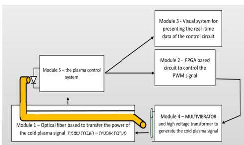
Figure 1 : Block diagram of the control system.
