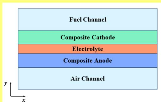
Fig. 2. Geometric model of SOEC unit.
