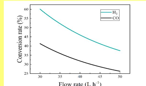
Fig. 4. The conversion rate of H<sub>2</sub> and CO with different inlet flow rate.
