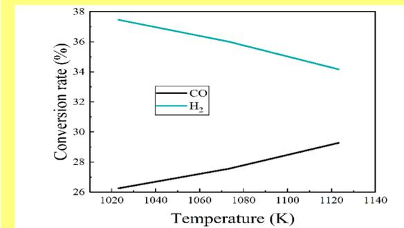
Fig. 5. The conversion rate of H<sub>2</sub> and CO with different temperature.
