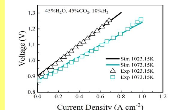
Fig. 3. Experimental and simulated polarization curves for cell at 1023.15K and 1073.15K.
