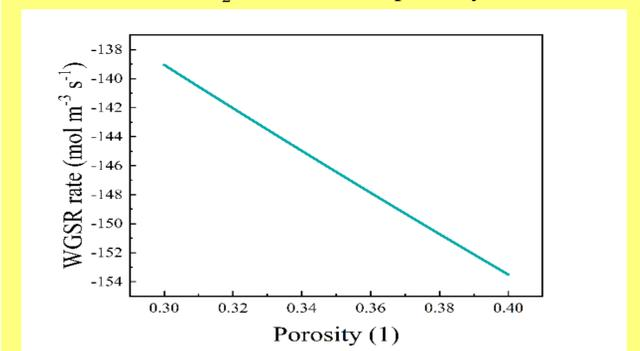
Fig. 7. The WGSR rate with different porosity.
