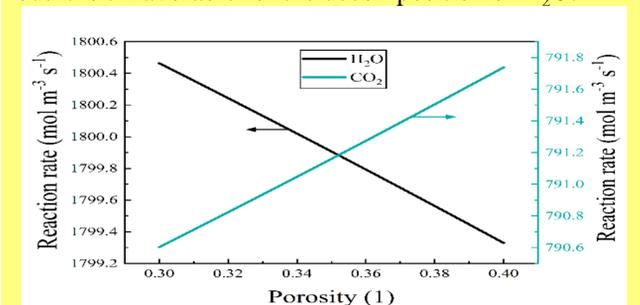
Fig. 6. The electrolysis reaction rate of H<sub>2</sub>O and CO<sub>2</sub> with different porosity.
