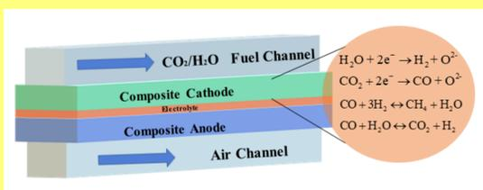
Fig. 1. Schematic diagram of co-electrolysis of H<sub>2</sub>O and CO<sub>2</sub> using SOEC.
