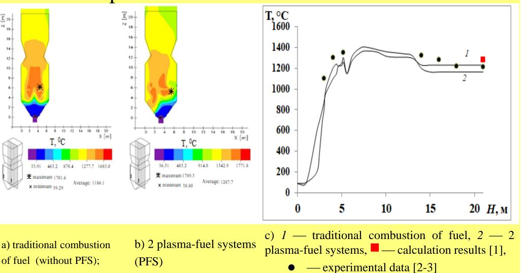
Figure 2 - Temperature distribution in the longitudinal section (a,b) and in height (c) of the combustion chamber of the BKZ-160 boiler
