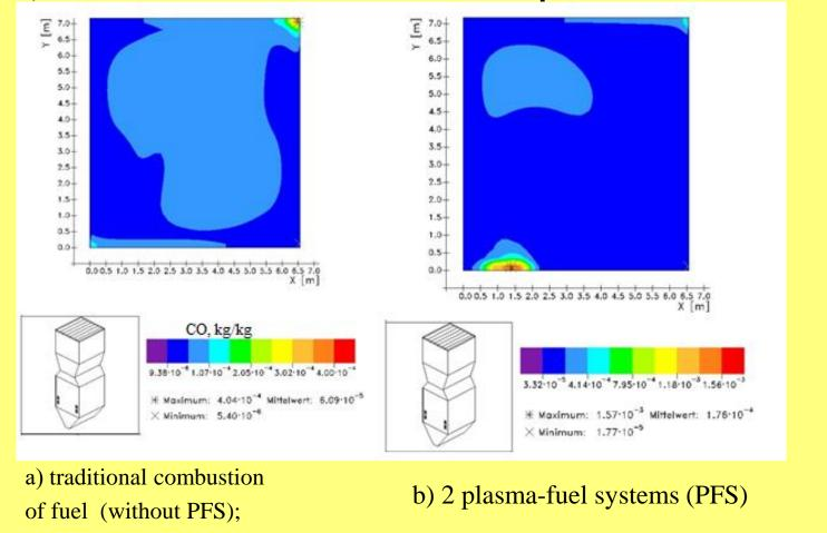
Figure 3 - Distribution of the carbon monoxide in the exit (a,b) and in height (c) of the combustion chamber of the BKZ-160 boiler
