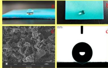
Fig.2. Superhydrophobic film on copper surface (a,b), microstructure of superhydrophobic film (c), static contact angle test diagram (d)
