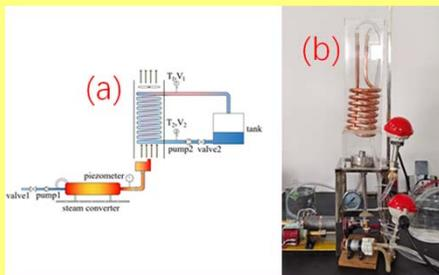
Fig.1. System schematic diagram, physical diagram
