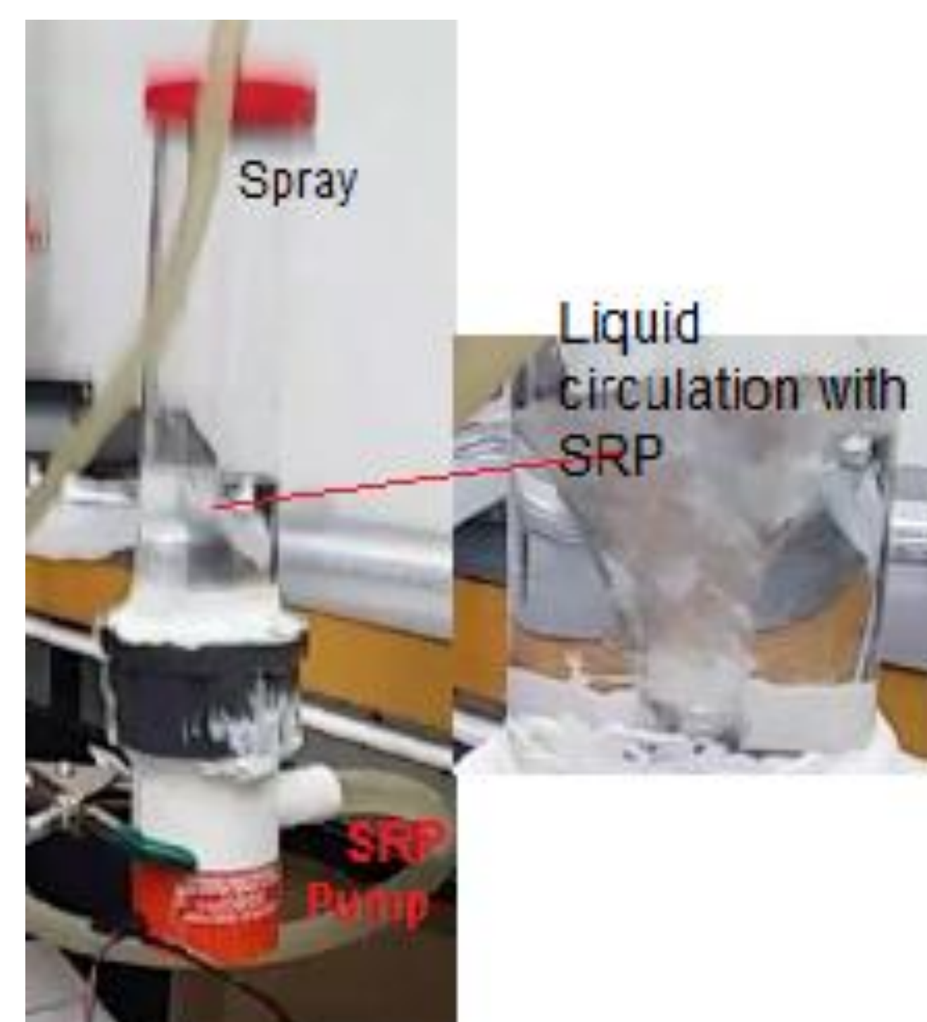
Fig.2 mixing and turbulence by SRP in the MEA solution created nano babbles of CO 2 with high area surface that improve the physical and chemical interaction exponentially
